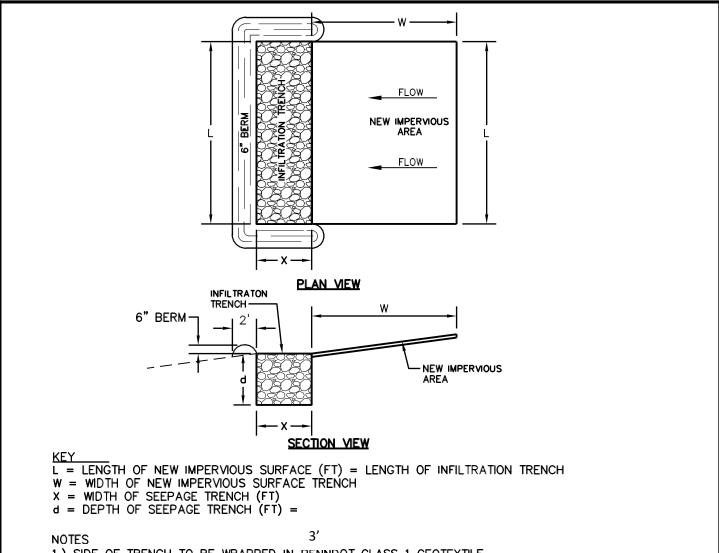
1.) SIDE OF TRENCH TO BE WRAPPED IN PENNDOT CLASS 1 GEOTEXTILE.
